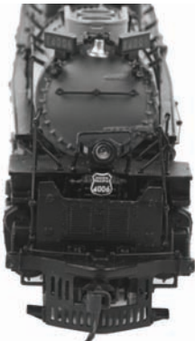
Engine Coupler Installed Front View
