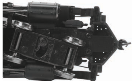
Engine Coupler Installed Underside View
