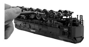
Next, remove brake shoe detail by gently prying and pulling up the part and set aside. Remove the screws holding down the rectangular chassis bottom cover. Carefully remove the cover, then carefully remove the 2 screws holding down the *gearbox* cover, set them aside and then stop. Don't do anything further until reading the next step completely.
