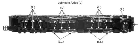
Lubricate Side Rods and Linkage (Both Sides) (LL)
