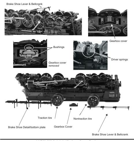
Now, very slowly and carefully lift the wheel set upward. Keep a close eye out for the driver springs as they sometimes stick to the bushings and lift out. If you drop one, you'll need some really good eyes or a magnet to find them. If they should lift out with the wheel set, carefully set them back into cavities from which they came.
