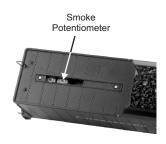
does in analog DC mode with the added benefit of being able to turn it on or off remotely. Pressing F12 on your DCC controller will toggle the smoke unit on and off again.
