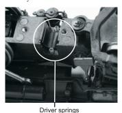
Drop the replacement wheel set into the chassis. Make sure the bushings are in the correct orientation. The small rectangular tabs on the front and rear must be upward (with the engine upside down) toward the chassis bottom cover.
